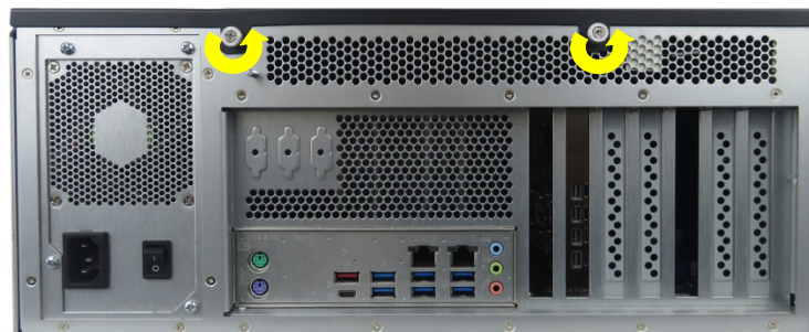
Figure 27: Loosening knurled screw on the rear side
